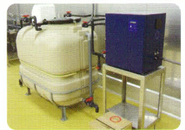
HOCL0.96t Floor, wall sterilization unit (Food processing factory)
